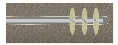
62. For all subsequent sets of perforations put into the casing, a frac plug and setting tool are included on the tool assembly. The frac plug provides hydraulic isolation of one set of perforations from the set of perforations that were punched and fractured previously.
