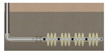
64. The main drawback with the "plug and perf" method is that each stage requires a new frac plug and perforating gun be run, meaning that the "spent" perforating gun must be pulled to the surface and replaced with a fresh gun and frac plug for the next stage to be stimulated. This increases the time required for completion, as well as the associated cost.
