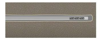
60. Once the perforating assembly has been lowered into the distal end of the wellbore (the toe), the operator moves and triggers each gun at selected intervals, punching holes through the cement and casing. This opens channels from the wellbore directly into the formation.
