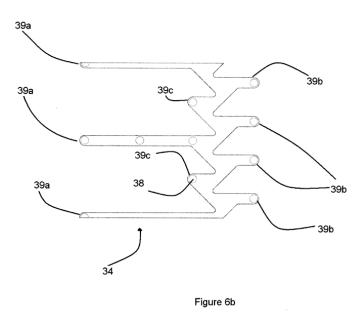
[397] Claim 4 indicates that it is dependent on Claim 1 and that the sliding member is an auto-J profile that is slidable against a pin to actuate the sealing member.
