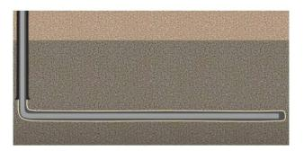
58. Plug and perf begins with a hole that has been cased and cemented, as shown below.
