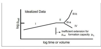
Appendix Figure 8. Log-log diagnostic plot for fracturing (Nolte, 1982).
