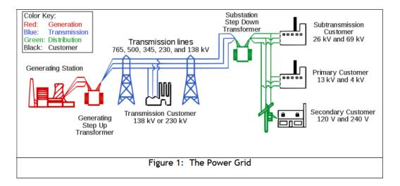
[19] Electricity is generated from resources such as coal and natural gas. Generating stations are commonly called power plants. Electricity is generated at power plants by electromechanical rotating machines, fueled by combustion or nuclear fission or, in the case of hydroelectric power generation, by water-driven turbines.
