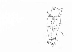
"a longitudinal opening providing access to the interior cavity, such that the articulated hydraulic boom can be positioned within the interior cavity of the sleeve"
