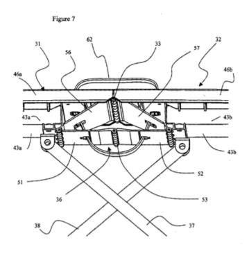
[236] Mr. Schuch says the tension rod means resists a tensile load placed specifically at its ends because it is connected at its outer ends to the overall structure. His opinion is based on there being no structural elements going across the interior of the tension rod plate to provide transverse loading.
