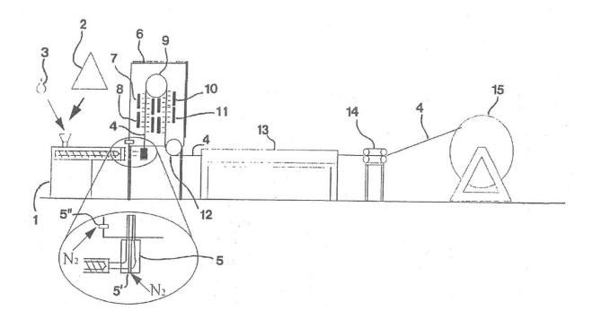
[26] The process, commencing at the left of the above diagram, is as follows: the peroxide (3) and polymer (2) are mixed in a hopper, and then enter the extruder. The extruded polymer pipe (4) then travels around a wheel and is directed 90° upwards through four IR zones (7, 8), it then
